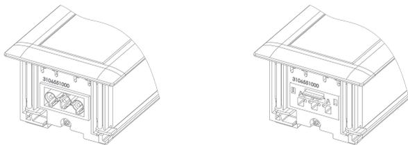
End cap with power input or output connector, depending on the surface thickness (max. 18 mm)
