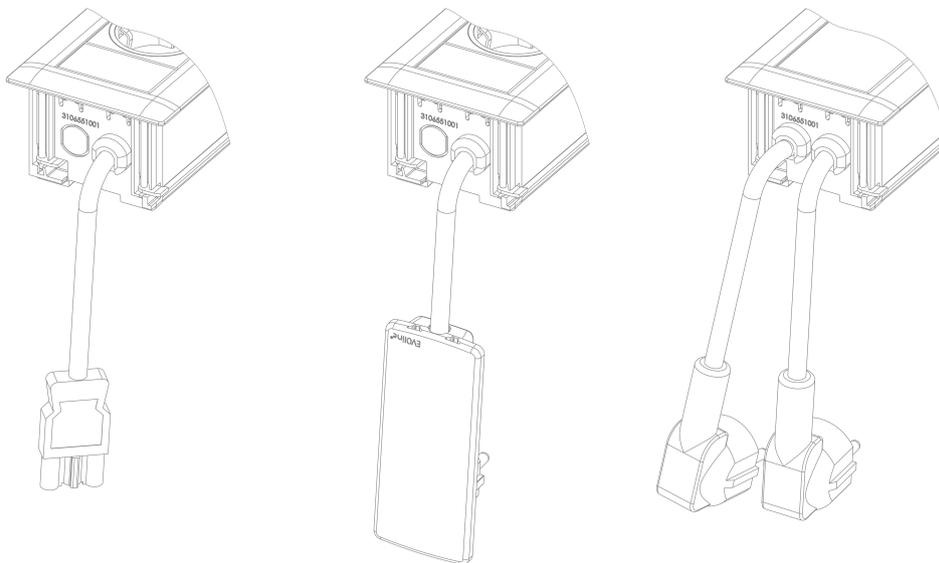
End cap with fixed power supply cable, depending on the surface thickness (max. 18 mm)
